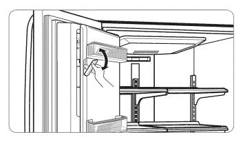
2. To remove the in-door ice bin, grip the front handle, slightly lift the lower part, and slowly pull out the bin as shown.
